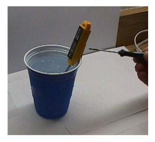
**DIGITAL PROBE CALIBRATION PROCEDURE FIGURE 1** THE DIGITAL PROBE CAN BE ATTACHED TO THE SIDE OF THE PLASTIC CUP DURING CALIBRATION BUT IT IS ALWAYS RECOMMENDED IT BE HELD WITH ONE HAND (NOT SHOWN) WHILE CALIBRATING TO PREVENT SPILLING THE CUP CONTENTS. THE METAL PART OF THE PROBE SHOULD NOT MAKE CONTACT WITH THE SIDES OR BOTTOM OF THE CUP. DeltaTRAK Technologies • 9260 Isaac Street, Ste. D • Santee, CA 92071 Tel: 800-390-0804 • Fax: (619) 596-4829 • E-mail: techsupport@deltatrak.com
